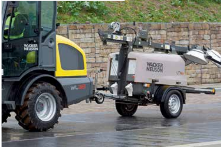
Trailer coupling for the transport of construction site equipment, such as a light tower.
