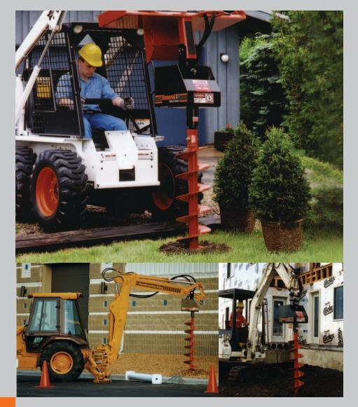
General's 671 DIG-R-TACH... derives power from the auxiliary hydraulic system of the carrier vehicle.
